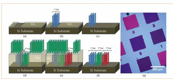
Figure 1: A three-step growth process of multi-color InGaN nanowire LEDs
