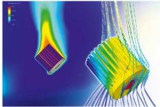
MechaTronix advanced pin fin coolers with 67 mm and 86 mm promise a performance gain of up to 30% compared to existing cooling platforms
