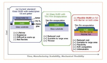
encapsulated devices. At the Holst Centre we are developing a low-cost, large-area thin film based barrier technology based on a SiN-organic-SiN stack which offers sufficient environmental protection to fulfill lifetime specifications of OLEDs / OPVs depending on the application. Most important is to keep in mind the scalability of the process for large area flexible lighting modules. The following diagram gives an overview of barrier encapsulation strategies vs cost.
