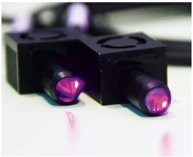
periodic system of elements that are used. UV LEDs basically belong to the same LED family as blue or green LEDs. They are GaN based and therefore the production process is quite similar. The LED color is defined by the amount and relation between the three elements of group III, Al (Aluminum), Ga (Gallium), In (Indium). The group V element, N (Nitrogen), always stays the same.
