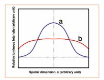
Figure 2: Schematics of one dimensional crosssection intensity profiles of LED lamp (a) and traditional lamp (b)
