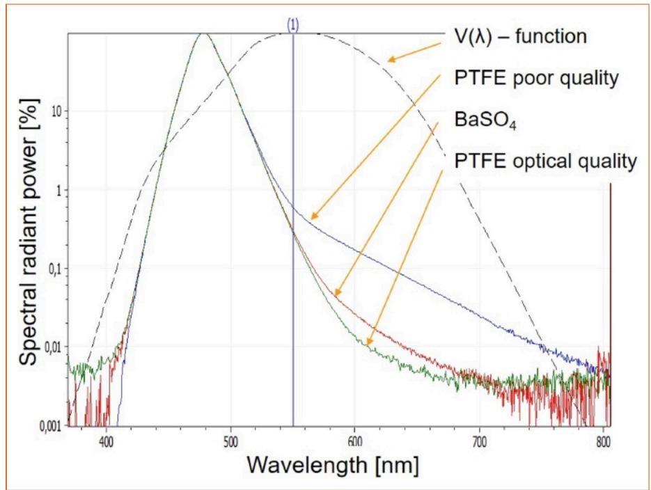
Figure 3: Blue LED measurements show higher fluorescence on the right flank for poor quality PTFE and lower fluorescence for the PTFE material with optical quality compared to barium sulfate (BaSO<sub>4</sub>).
