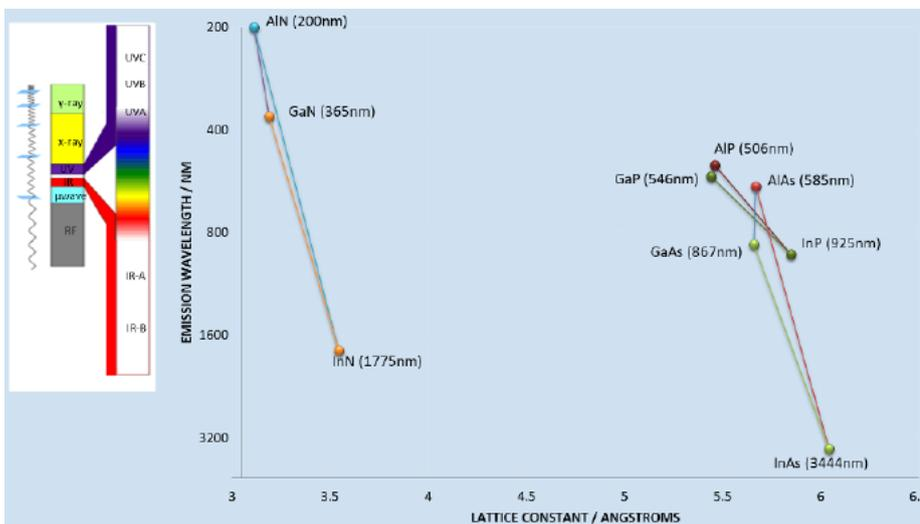
Figure 4: Group III-V Ternary Material System  $Al_xGa_yIn_zN$ ,  $Al_xGa_yIn_zP$  and  $Al_xGa_yIn_zAs$
