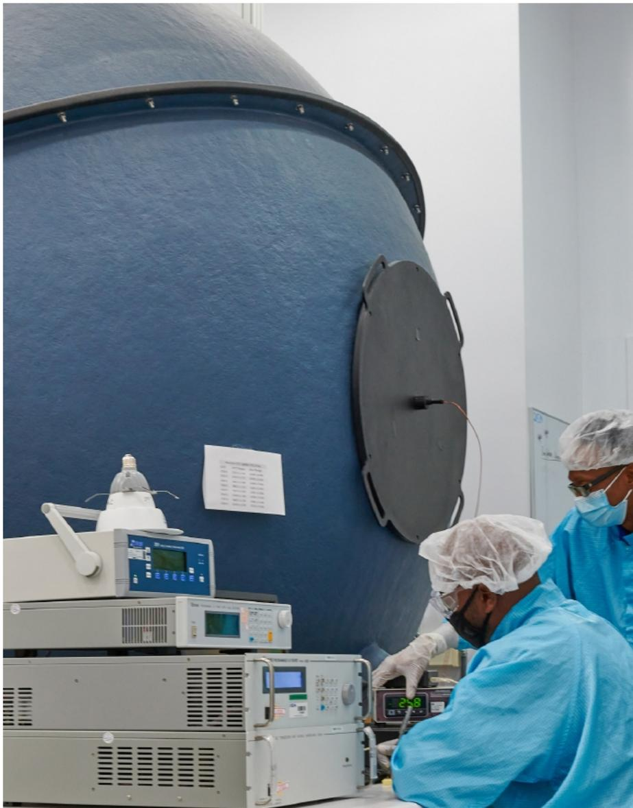
Figure 2: A 3-meter integrating sphere for fixture analysis in Cree LED labs.
