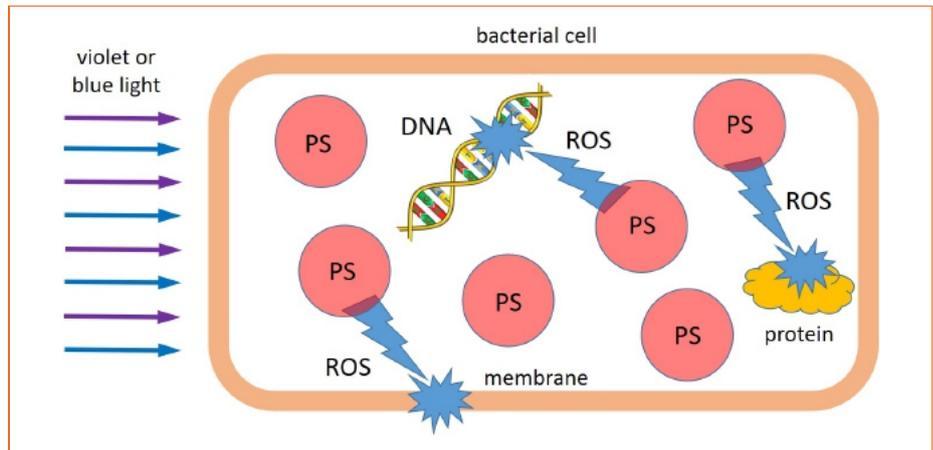
Figure 2: Scheme of the disinfection mechanism of blue and violet (purple) light for bacteria [2] (PS: Photosensitizer, ROS: Reactive Oxygen Species, DNA: Deoxyribonucleic acid).
