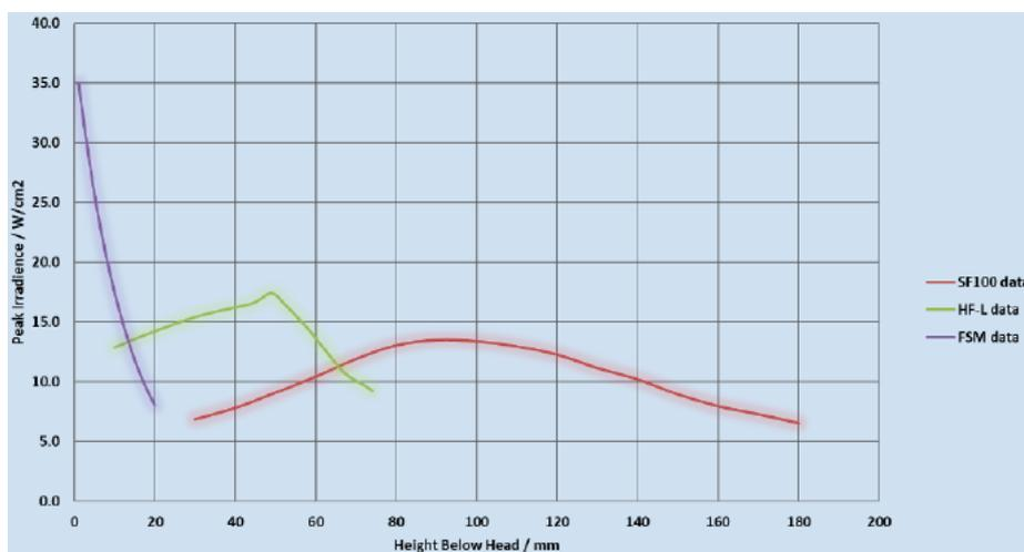
Figure 2: UV Output FSM, HF-L and SF100 UVed2 Reflector Systems (385 nm to 395 nm) measured with EIT LEDR-R395.
