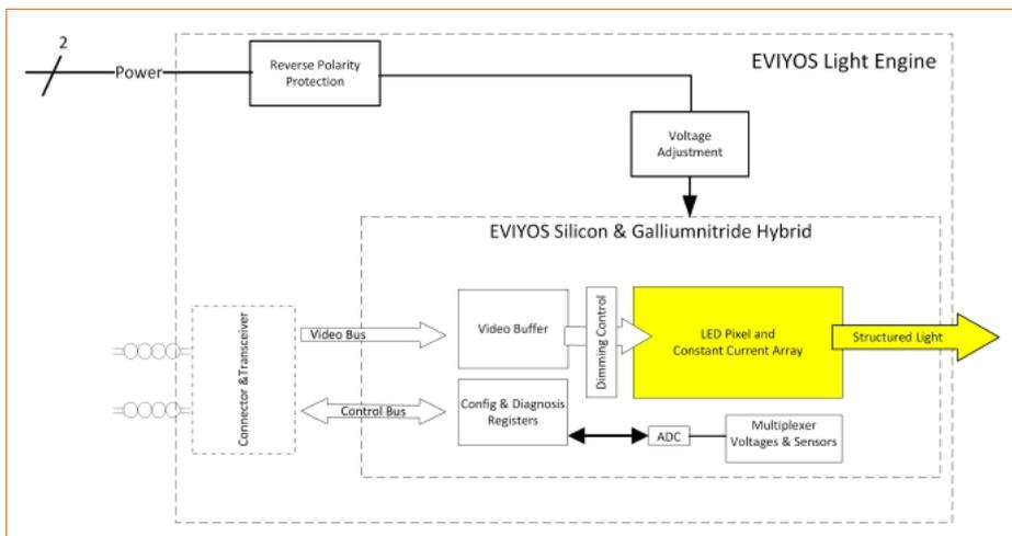
Figure 4: Eviyos LED pixel array light engine.
