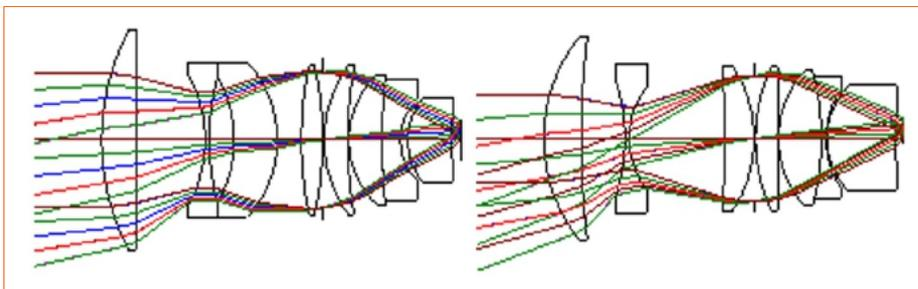
Figure 7: Structure of the lens systems. Small field of view (left) compared to a large field of view (right).
