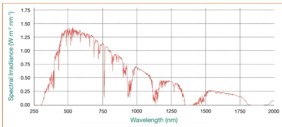
Figure 1: Air Mass 1.5 Global Reference Spectrum.
