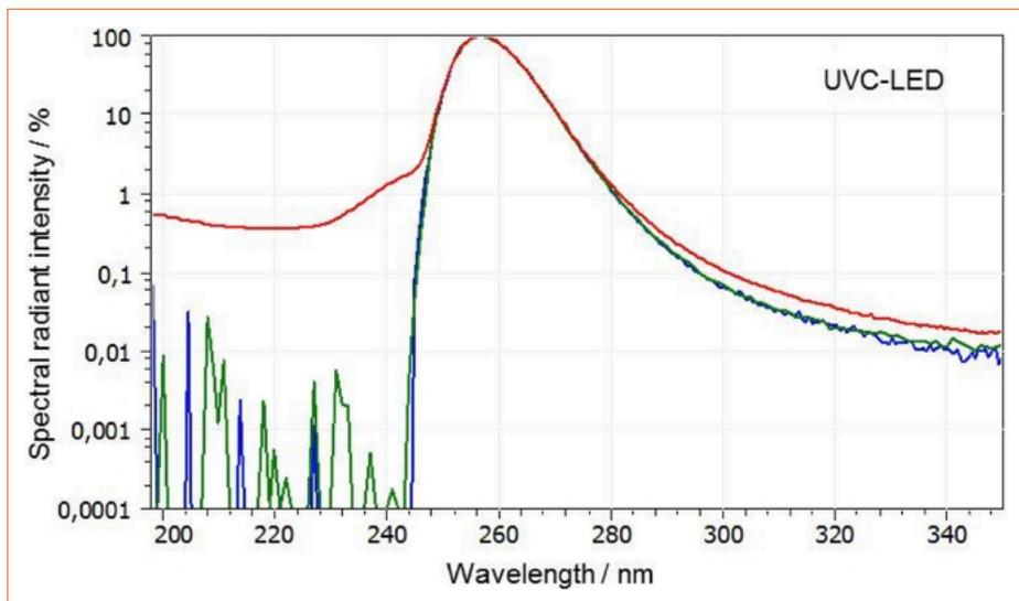
Figure 1: Logarithmic display of the spectra of a UVC LED with (blue) and without (red) stray light correction of an array spectroradiometer, measured with a double monochromator (green).
