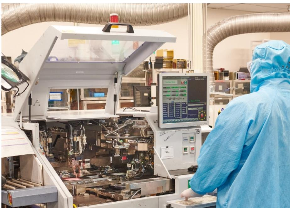
Figure 3: Die bonder in a Cree LED Pilot Production Facility.
