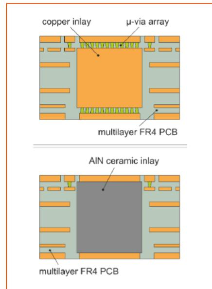
Figure 6: Multilayer PCB technologies with copper or aluminum nitride inlays.
