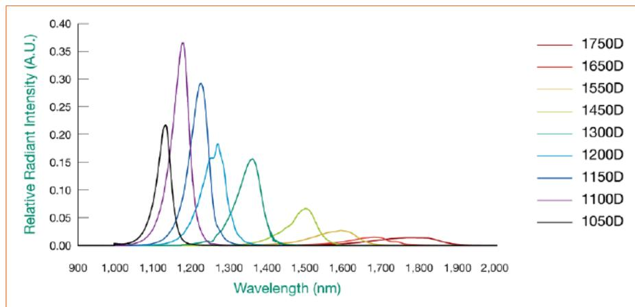
Figure 4: Epitex D Series SWIR LEDs.
