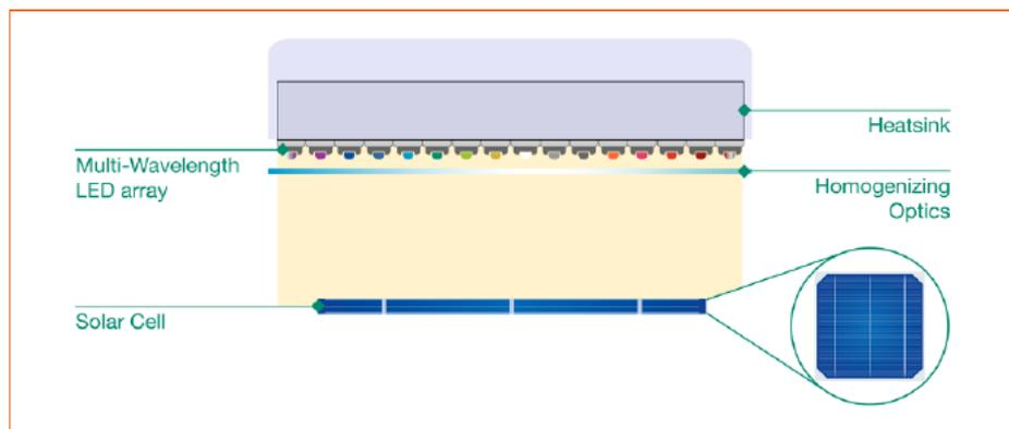
Figure 5: Concept schematic of an LED Solar Simulator for solar cell testing.
