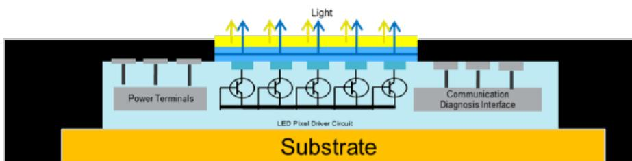
Figure 2: Concept of the light source device. The GaN-LED array is placed on top of the pixel driver IC in the package.
