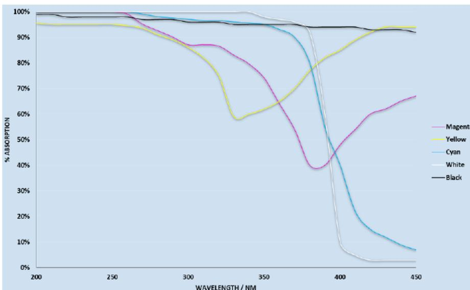
Figure 5: % Absorption of common process pigments in the UV region.
