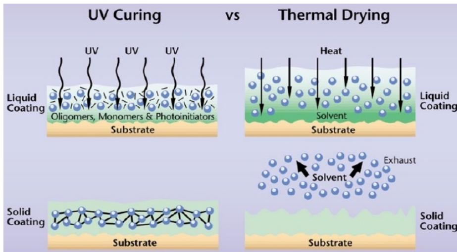
Figure 1: Comparison between UV Curing and Thermal Drying.
