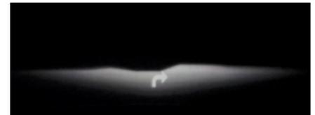
Figure 1: The screenshot from the setup in the ams OSRAM laboratory shows the combination of the classic glare free high-beam function with the projection of certain symbols.
