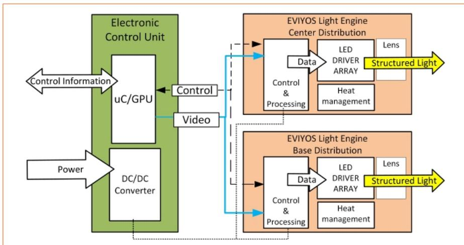
Figure 3: Architecture for one headlamp consisting of two Eviyos light engines and one ECU.
