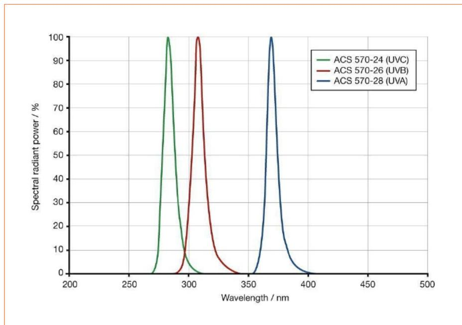
Figure 6: Typical spectra for UV-LED calibration standards.
