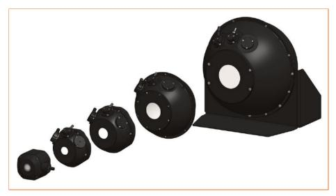
Figure 2: Integrating spheres made of optically pure polytetrafluoroethylene (PTFE) for low-fluorescence measurements of the radiant flux in the UV.
