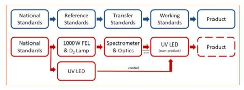
Figure 4: Calibration chain at national metrology institute (blue) and at Instrument Systems (red).
