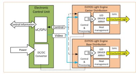
Figure 3: Architecture for one headlamp consisting of two Eviyos light engines and one ECU.
