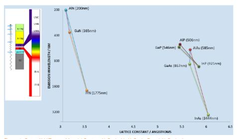
Figure 4: Group III-V Ternary Material System Al<sub>x</sub>Ga<sub>y</sub>In<sub>z</sub>N, Al<sub>x</sub>Ga<sub>y</sub>In<sub>z</sub>P and Al<sub>x</sub>Ga<sub>y</sub>In<sub>z</sub>As
