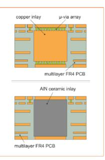
Figure 6: Multilayer PCB technologies with copper or aluminum nitride inlays.
