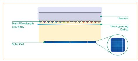
Figure 5: Concept schematic of an LED Solar Simulator for solar cell testing.
