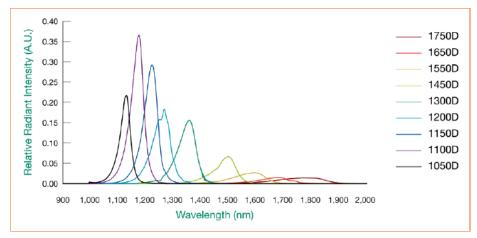
Figure 4: Epitex D Series SWIR LEDs.
