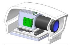
Figure 5: Cross section of a Dual System with one Unit.
