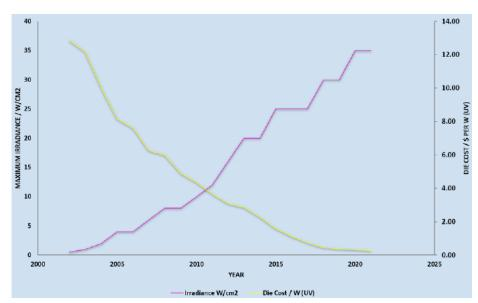
Figure 6: Evolution of UV performance and die costs for 395 nm.
