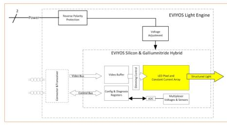
Figure 4: Eviyos LED pixel array light engine.
