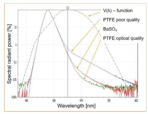
Figure 3: Blue LED measurements show higher fluorescence on the right flank for poor quality PTFE and lower fluorescence for the PTFE material with optical quality compared to barium sulfate (BaSO<sub>4</sub>).
