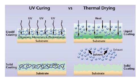
Figure 1: Comparison between UV Curing and Thermal Drying.
