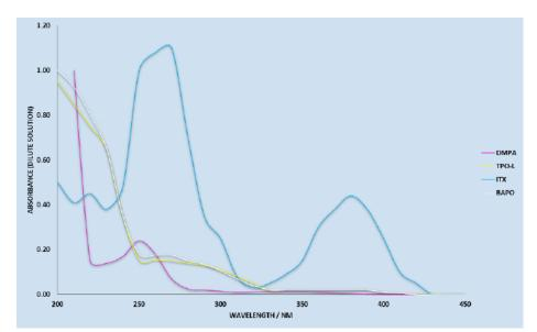
Figure 3: Absorbance of common UV LED photoinitiators in the UV region.
