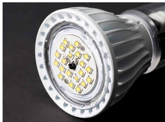
Figure 5: LED module with 21 Lumileds LUXEON TX white high-power LED chips mounted on a ceramic circuit board
