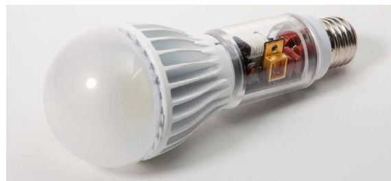
Figure 4: LED lamp in E27 bulb form factor with a power converter based on a GaN HFET in TO-220 package (section containing the power converter extended for demonstration purposes)
