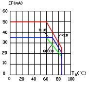
MAXIMUM FORWARD DC CURRENT VS, AMBIENT TEMPERATURE.
