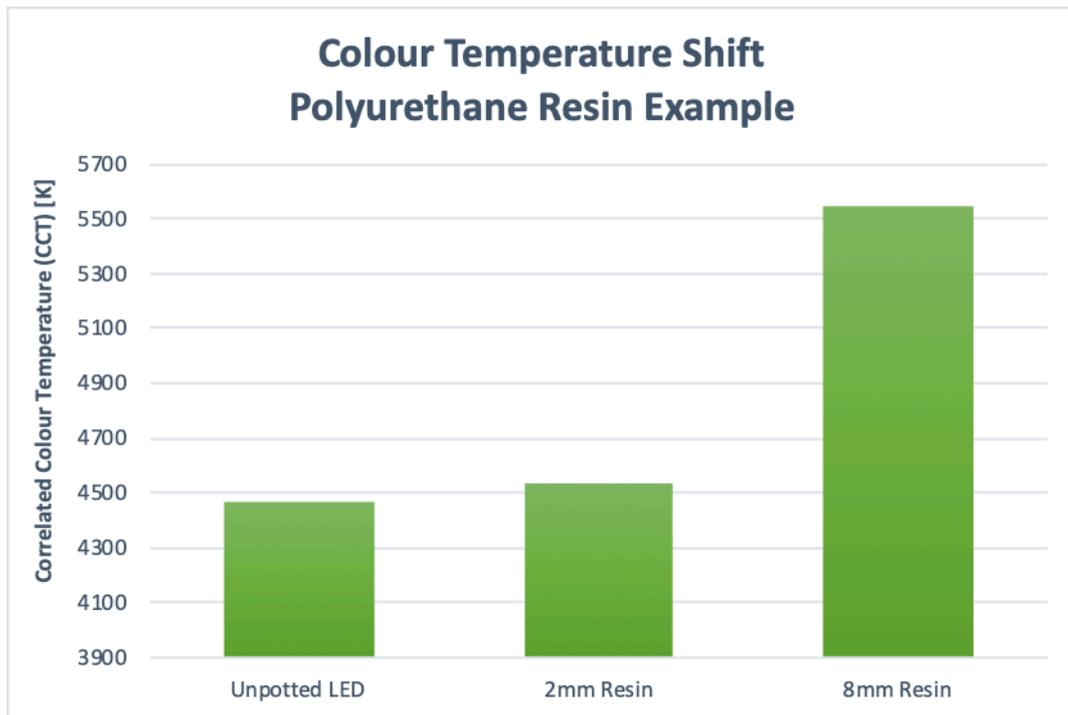
*Graph 5 – Effect of resin thickness on colour temperature shift*
