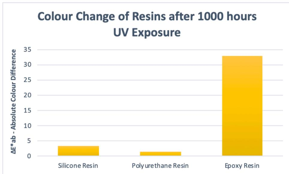
*Graph 3 – Comparison of standard resin chemistries after 1000 hours exposure to UV light*
