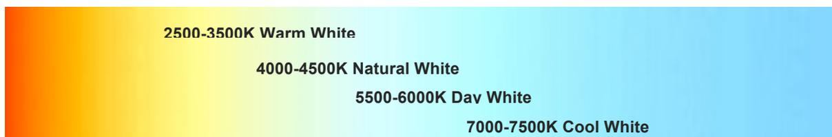
*Image 1 – Typical Colour Temperature Bands for LEDs*
