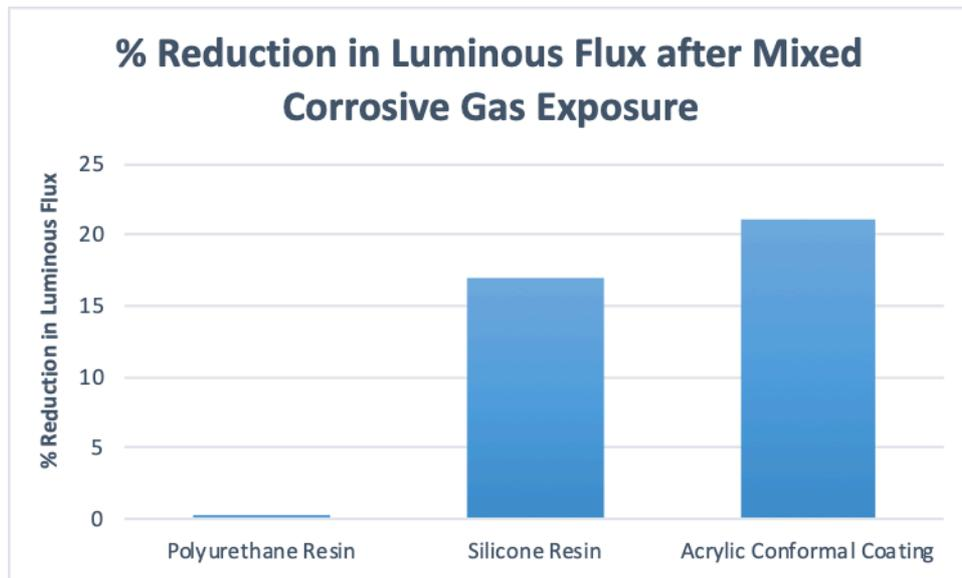
*Graph 4 – Change in luminous flux after exposure to mixed corrosive gas*
