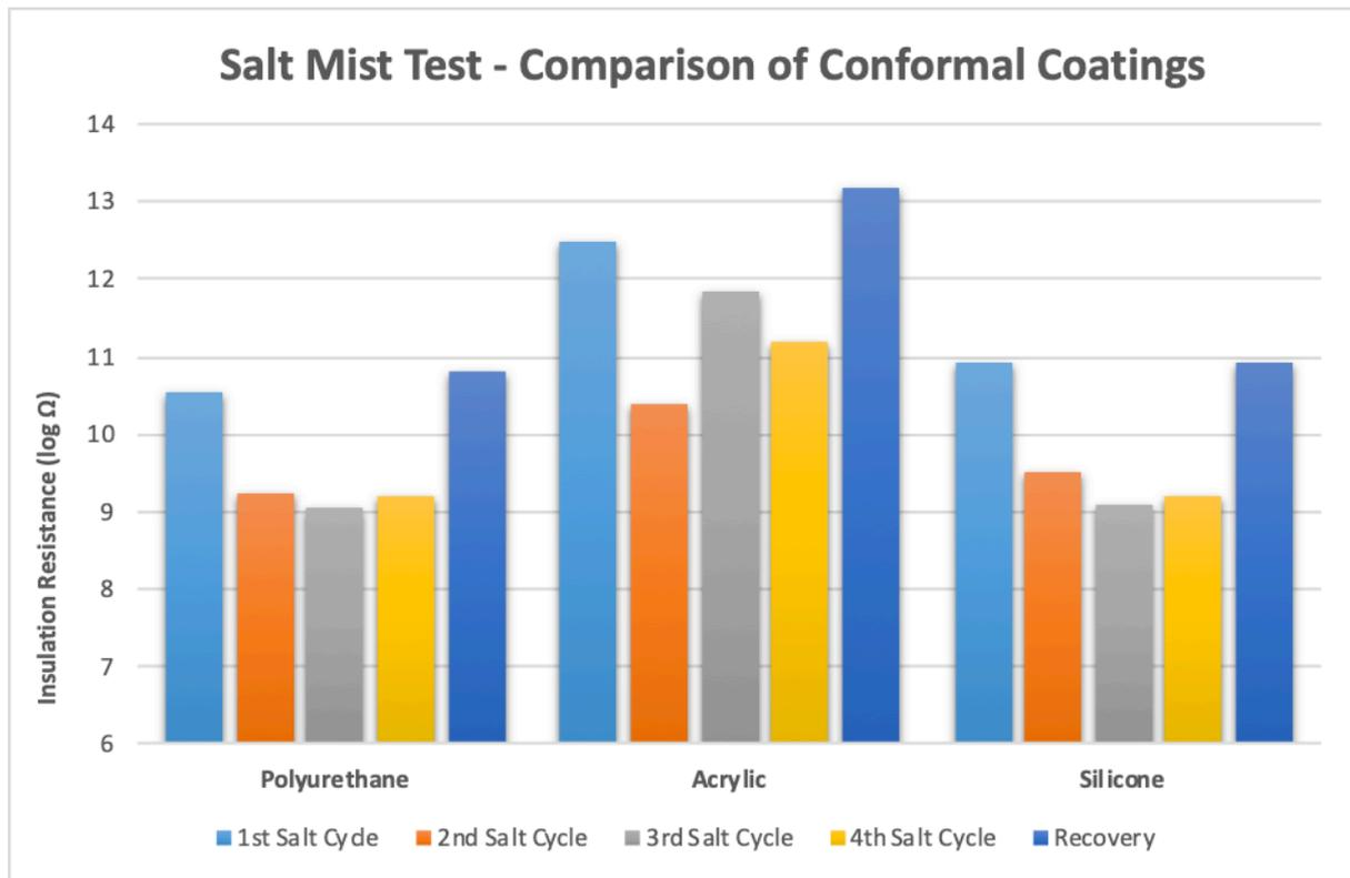
*Graph 1 – Comparison of conformal coating performance in a salt mist environment*
