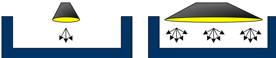
Figure 4. Effect of luminaire size and beam angle
