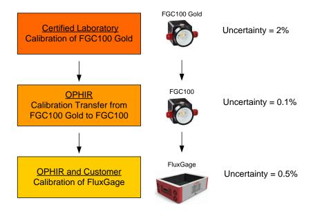
Figure 3. FluxGage calibration chain
