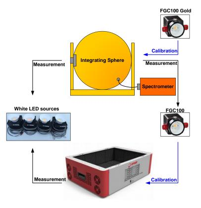
Figure 6. Experimental verification scheme
